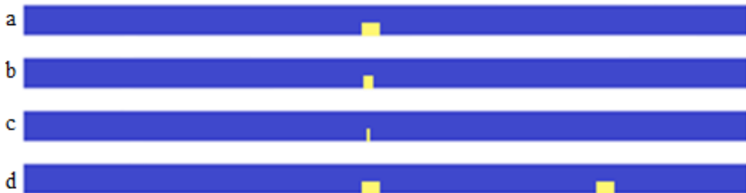
Figure 5. (a) 0.3 mm wire-cut crack (b) 0.1 mm wire-cut crack (c) 0.03 mm welding crack (d) two 0.3 mm wire-cut cracks
