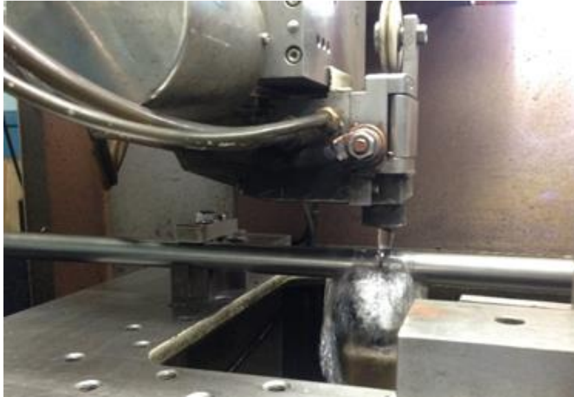
Figure 3. Enlarged view of 0.1 mm wire-cutting process
