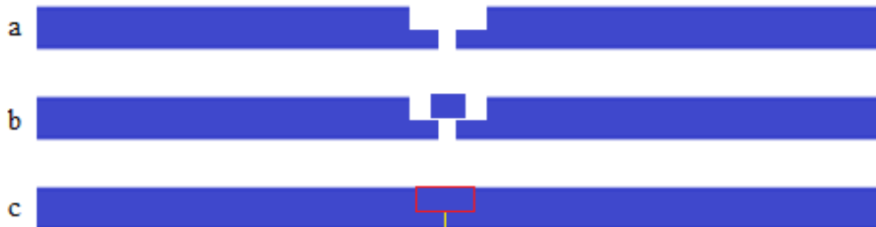
Figure 4. Procedure of welding crack (a) two halves milled (b) donor piece (c) welded together (red lines) and yellow representing 0.03 mm welding crack
