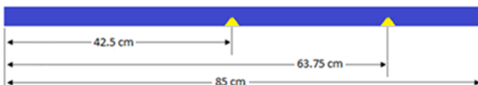
Figure 2. Diagram of shaft with cutting dimensions
